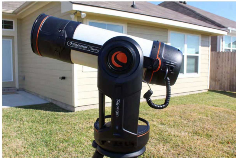
Image 6 – The mount has a handle on the arm and two on the base for gripping when carrying the mount and attaching it to the tripod top plate. The power switch and power cord receptacle are located below the arm. There is a power light on the arm below the word "origin". Note the cable that connects the OTA to the mount. The telescope will not operate without the cable in place.
