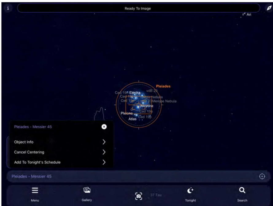
Image 38 – The orange circle in the planetarium window contains the current object the Origin telescope is pointing at. The orange rectangle shows the portion visible on the camera's sensor.
