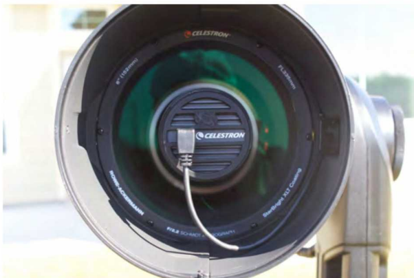
Image 2 – The onboard camera presents a central obstruction 63 mm in diameter (41%).
