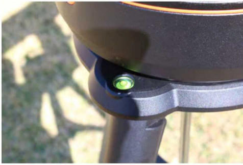
Image 5 – There is a built-in bubble level on the top plate of the tripod, which is visible with the mount attached. The telescope should be level during operation.
