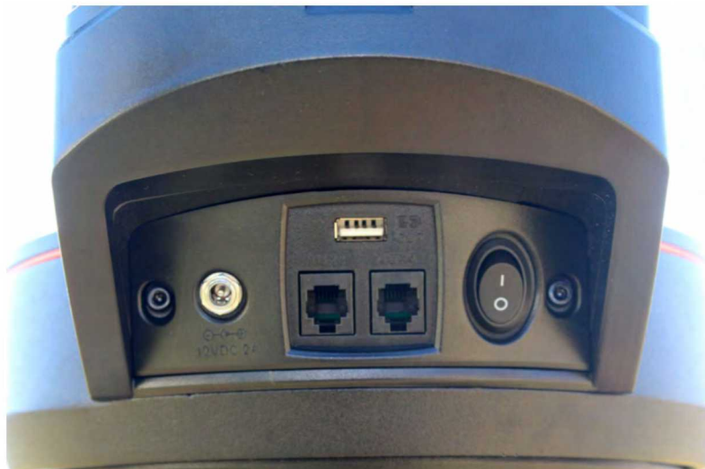
Image 8 – Close-up view of the power panel. From left to right are the power cord receptacle, two additional auxiliary port, a USB port to power a phone or tablet, and the on/off switch.
