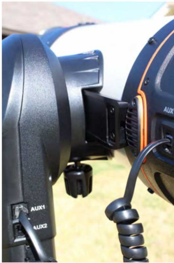
Image 7 – A dovetail plate attached to the OTA is shown here clamped into the single arm of the mount. Note the auxiliary jacks on the mount and OTA.
